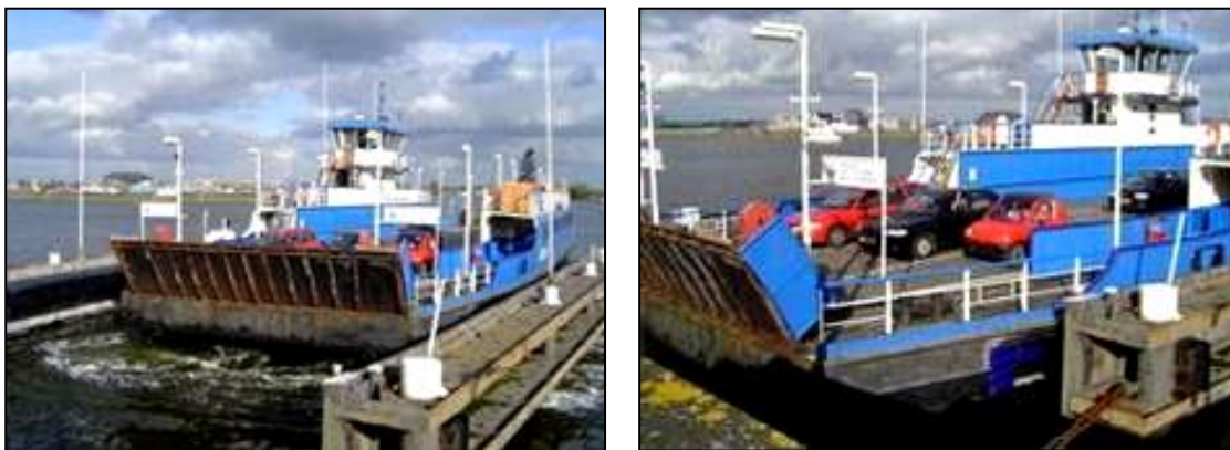
Figure 6.26 – Car Ferry capable of transporting 40 Cars or some 850 PAX
