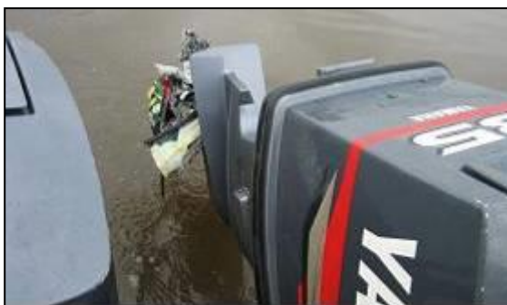
Figure 6.47 – Plastic Bags in an Outboard Propeller
