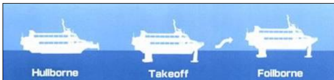
Figure 6.43 – Different Stages for a Hydrofoil Vessel [source: Source: Kawasaki Jetfoils]
