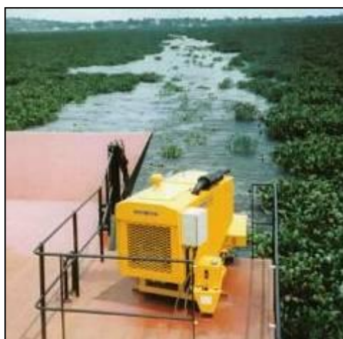
Figure 6.49 – Z Drive System in Operation on Lake Victoria
