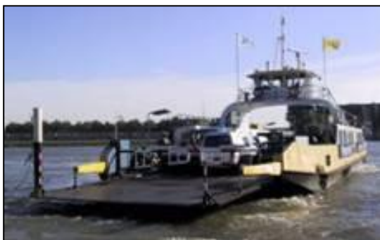
Figure 6.24 – Car Ferry capable of transporting some 15 Cars
